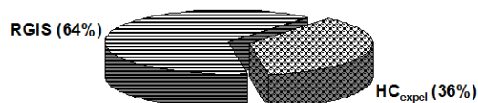
Fig 7: Gas Expelled and Retained in the Ranikot Shale for the Southern Indus Basin
