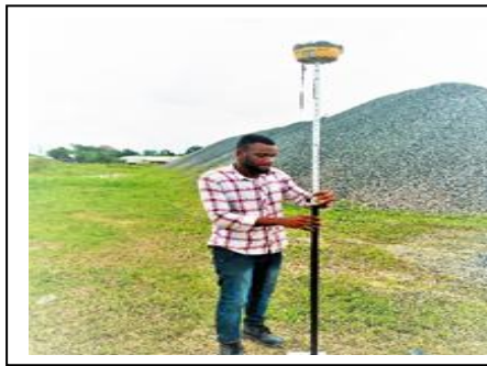
Fig. 5: Coordination of the GCPs with GNSS Receiver
