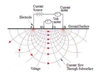
Fig 2: Two current and two potential electrodes on the surface of ground of resistivity (Source: Elhag, 2016).
