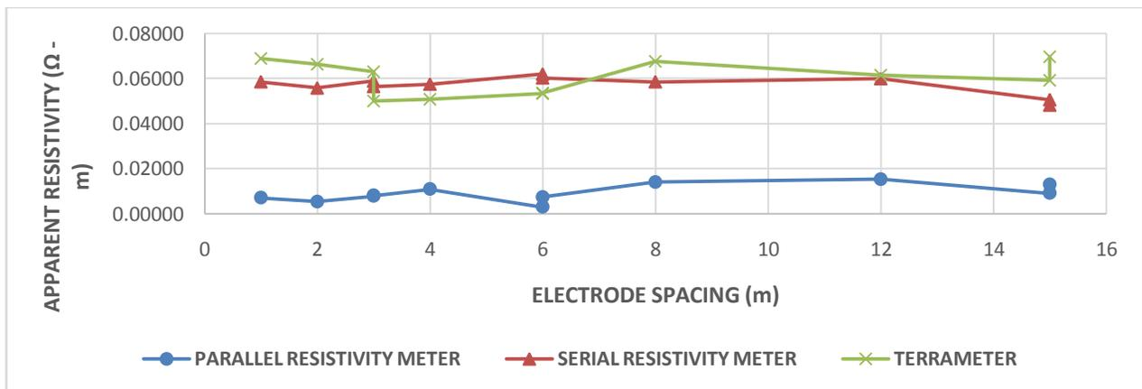
Figure 8: Profile Analysis of the resistivity meters for site five
