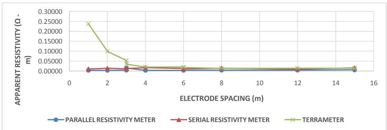
Figure 9: Profile Analysis of the resistivity meters for site six
