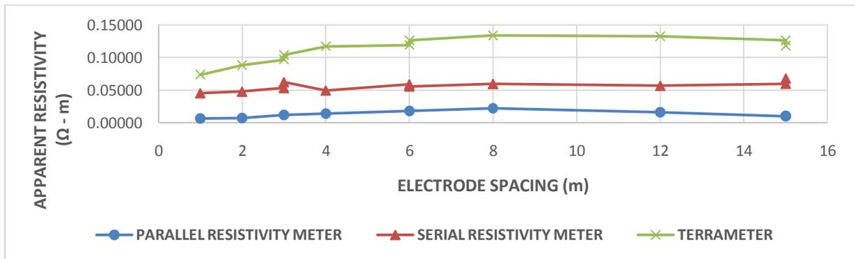
Figure 5: Profile Analysis of the resistivity meters for site two
