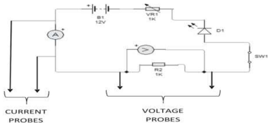
Figure 3: Circuit layout of a parallel resistivity meter
