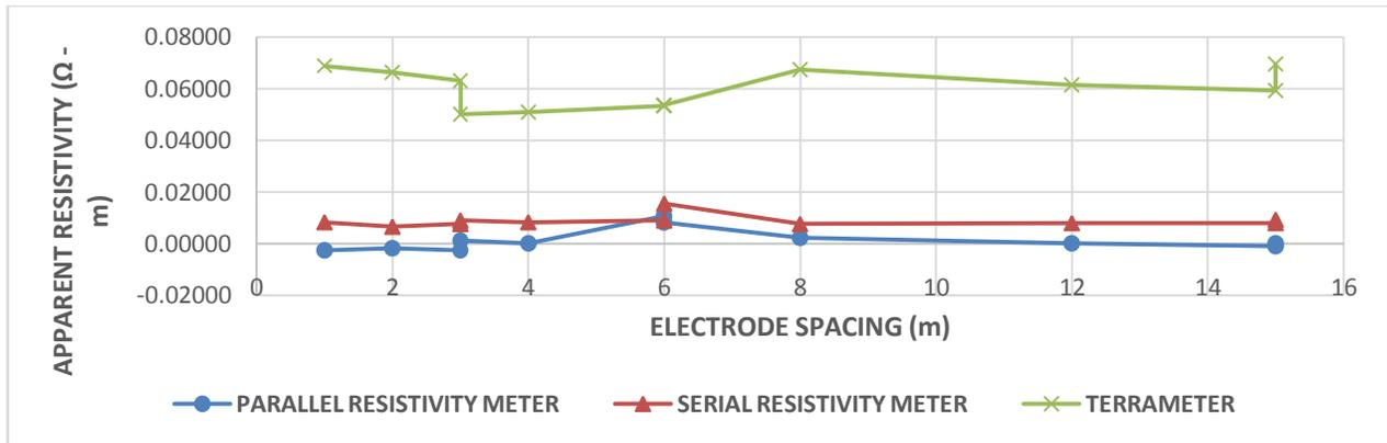
Figure 7: Profile Analysis of the resistivity meters for site four
