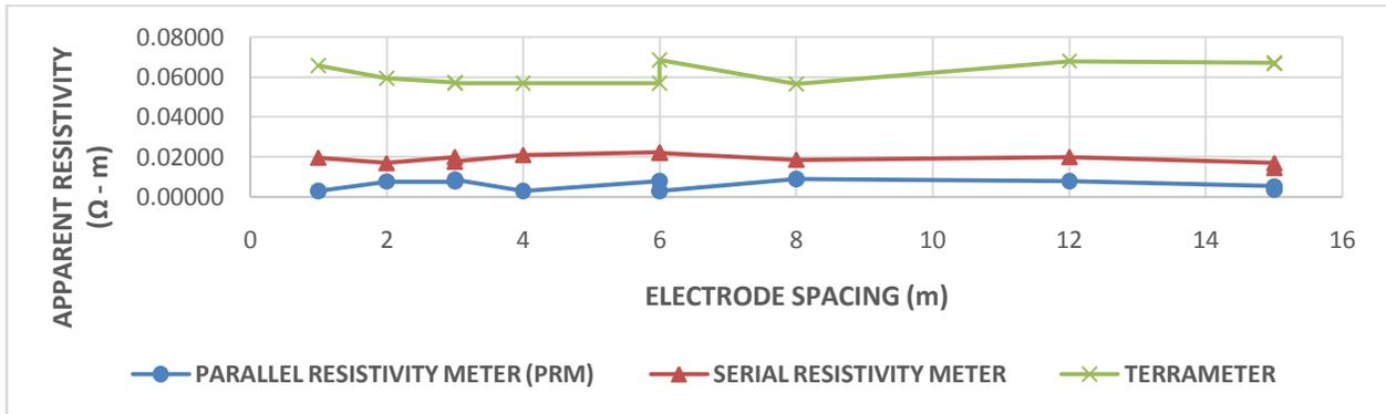
Figure 4.: Profile Analysis of the resistivity meters for site one
