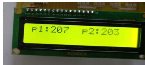
Fig.6 Leak location on LCD
