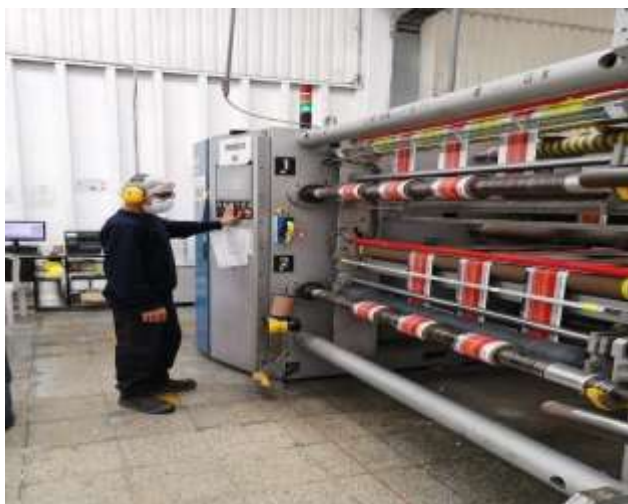
Fig. 2 Cutting Machine Used for Initial Inspection and Cleaning
