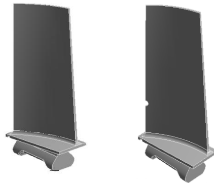
Fig 1: Twisted turbine blade with and without notch.
