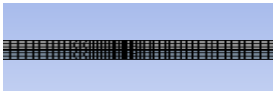
Fig.4: Refine mesh at the crack tip
