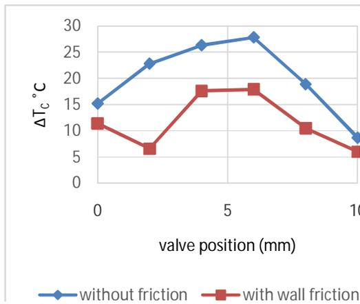
Fig. 8 Effect of wall friction on temperature separation at inlet pressure 85 psi
