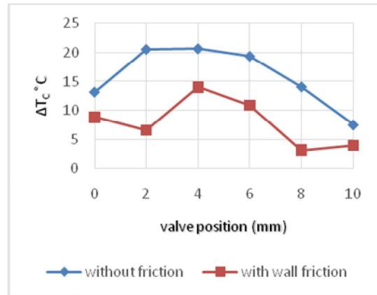
Fig. 5 Effect of wall friction on temperature separation at inlet pressure 50 psi
