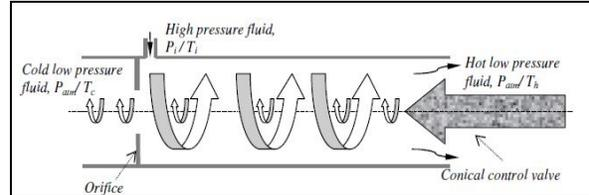
Fig. 1 Schematic diagram of Counter flow vortex tube
