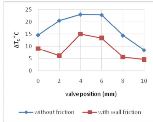
Fig. 6 Effect of wall friction on temperature separation at inlet pressure 60 psi
