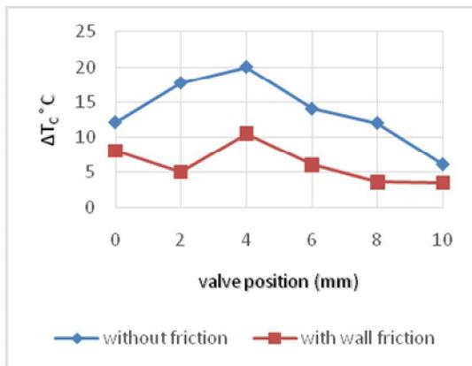
Fig. 4 Effect of wall friction on temperature separation at inlet pressure 40 psi
