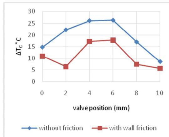
Fig. 7 Effect of wall friction on temperature separation at inlet pressure 75 psi
