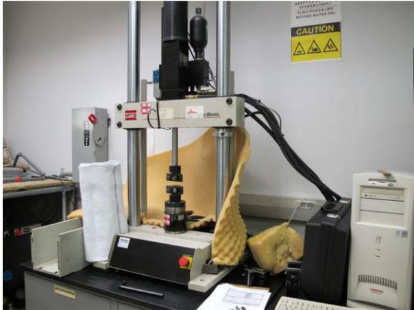
Figure 12: Universal Tensile Testing Machine
