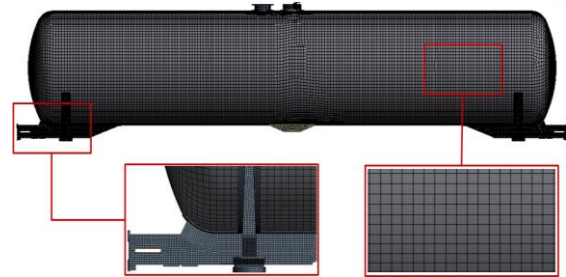
Figure 4. Detail of the mesh in the tank and stub sill.
