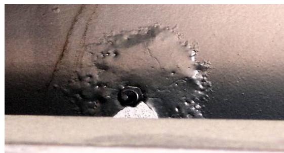
Fig (15) - Filiform Corrosion in an Aircraft Part.
