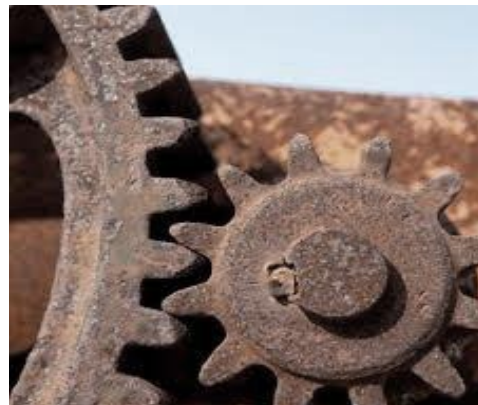
Fig (1) - Corrosion Affected Gears
