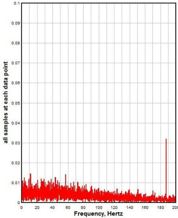
Fig. 3 Fast Fourier Transform (FFT) of the Hotwire Data at 1D Downstream of the Jet Exit
