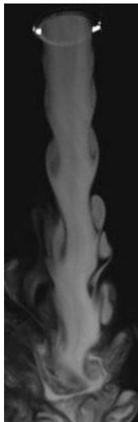
**Fig. 7 : Flow Visualization of an Axisymmetric Turbulent Jet at Steady State**
