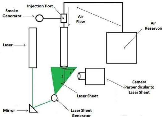
Fig. 1 Flow Visualization Setup
