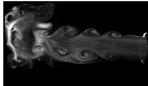
**Fig. 9 : Flow Visualization of an Axisymmetric Turbulent Jet at the Transient Start Following the Initial Vortex**
