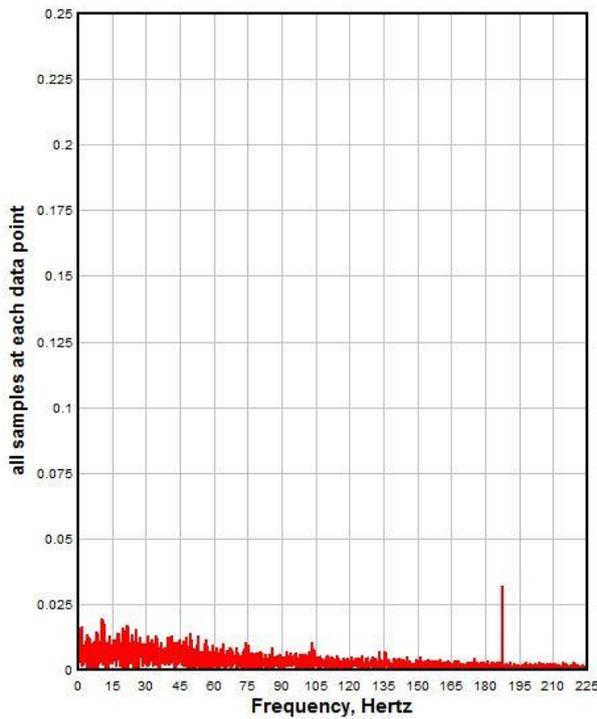
Fig. 4 Fast Fourier Transform (FFT) of the Hotwire Data at 2D Downstream of the Jet Exit
