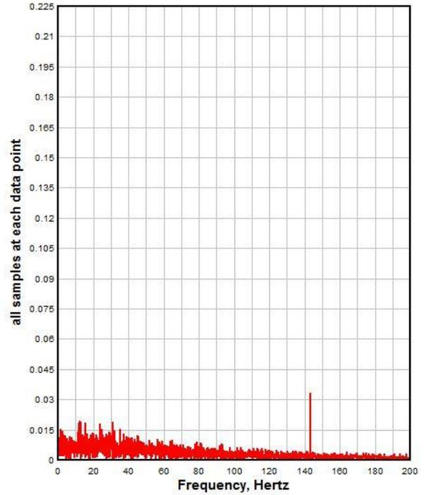
Fig. 5 Fast Fourier Transform (FFT) of the Hotwire Data at 3D Downstream of the Jet Exit
