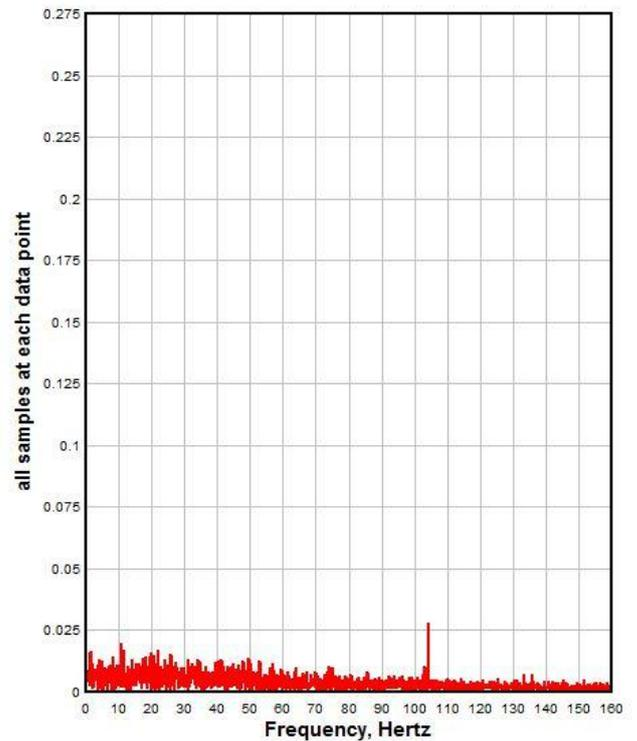
Fig. 6 Fast Fourier Transform (FFT) of the Hotwire Data at 4D Downstream of the Jet Exit
