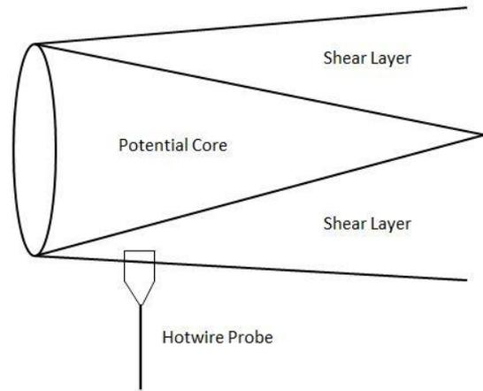
Fig. 2 Position of Hotwire Probe
