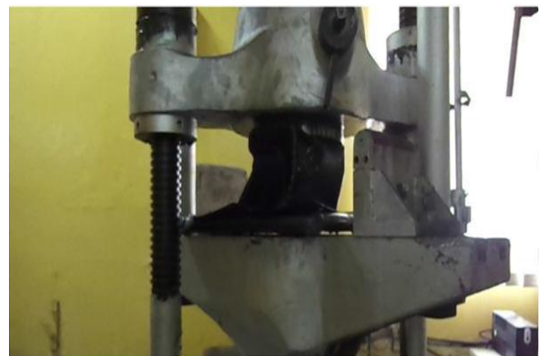
Fig. 4: Midway Crushing of Impact Attenuator.
