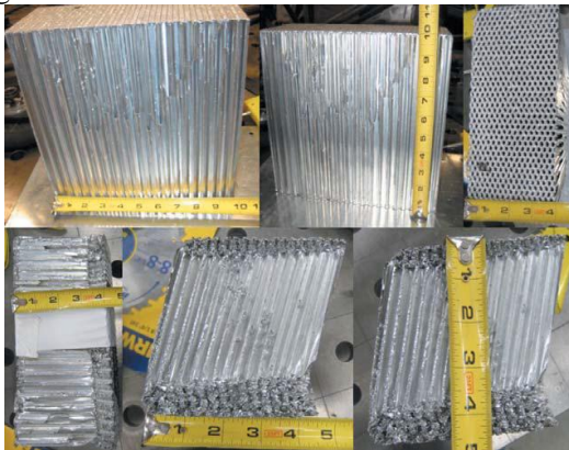
Fig. 2: Impact Attenuator Before and After Testing.
