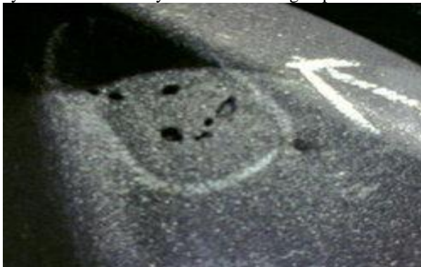
Figure 6: The Shrinkage Porosity Defect in the Feeder after Cutting it with Center Plane.
