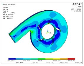
According to this the minimum value for stress is 27.2514  $N/mm^2$  and maximum value is 3385.94  $N/mm^2$
