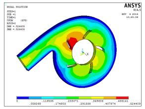
According to this the minimum value for displacement is 0.116535mm and maximum value is 0.524409mm
