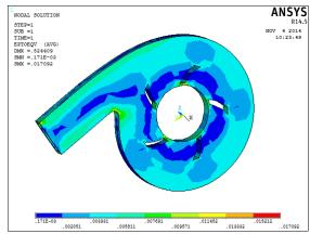
According to this the minimum value for strain is 0.171E-03 and maximum value is 0.17092
