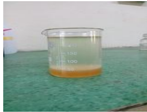
Fig.2: Bio Diesel at Top & Glycerol at bottom
