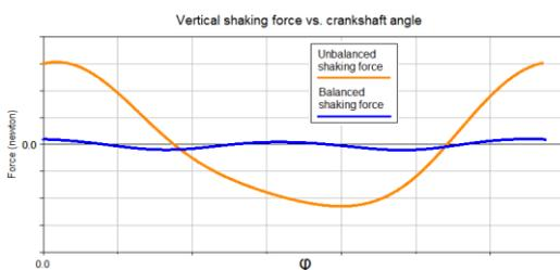
**Figure 9 Balanced and Unbalanced Vertical Shaking Force.**
