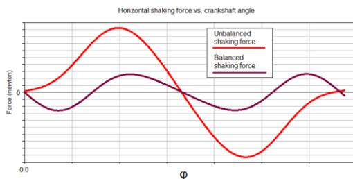
**Figure 8 Balanced and Unbalanced Horizontal Shaking Force.**
