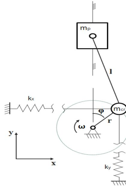
Figure 1 Spring Balanced Slider-Crank Mechanism
