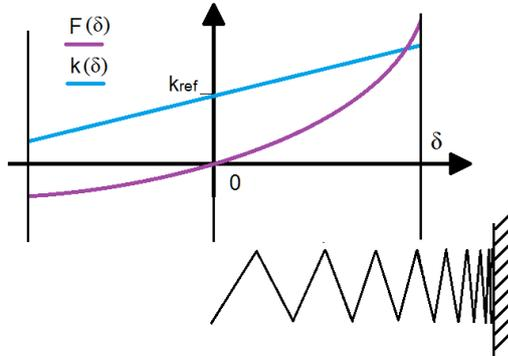
Figure 5 Typical Progressive Spring Curve
