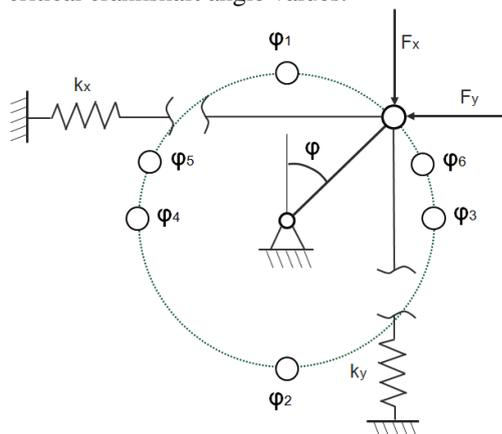
Figure 2 Simplified Model of the Spring Balanced Slider-Crank Mechanism
