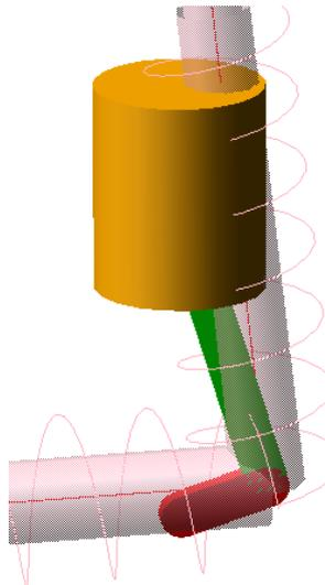
**Figure 7 Multibody Model of Spring Balanced Slider-Crank Mechanism**
