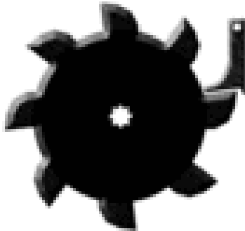
Fig 3. Ratchet With Round Gear and Pivot
