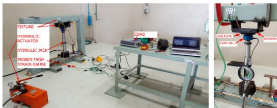
Fig. 7. Fixture And Experimental Set Up
