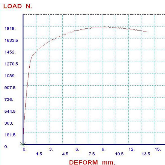
Fig.6. Load Vs. Deformation Curve of External Bend Test
