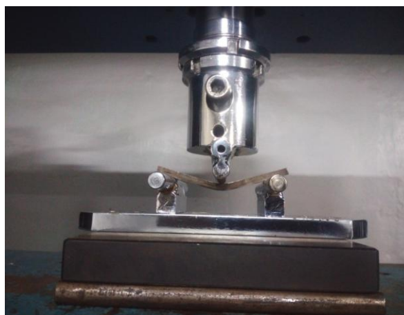
Fig.3. Experimental Three Point Bend Test
