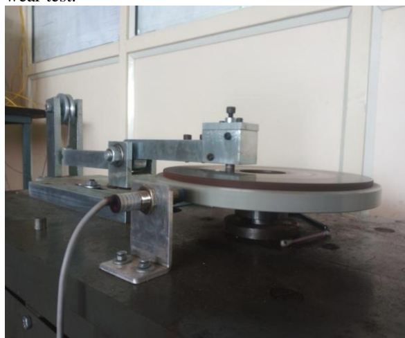
Fig.4. Experimental Wear Test on Pin-on-Disk Tribometer
