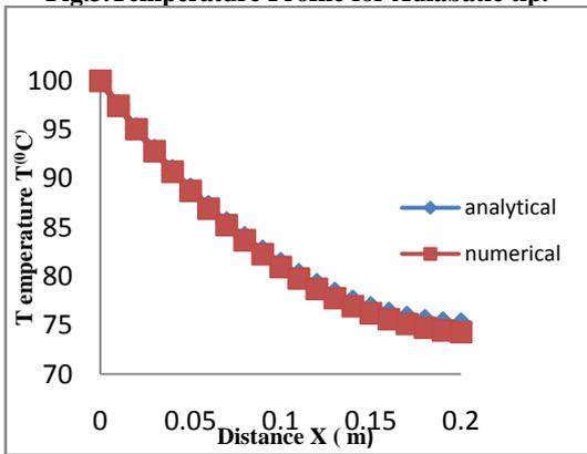
Fig.4. Temperature Profile for Convective Tip.
