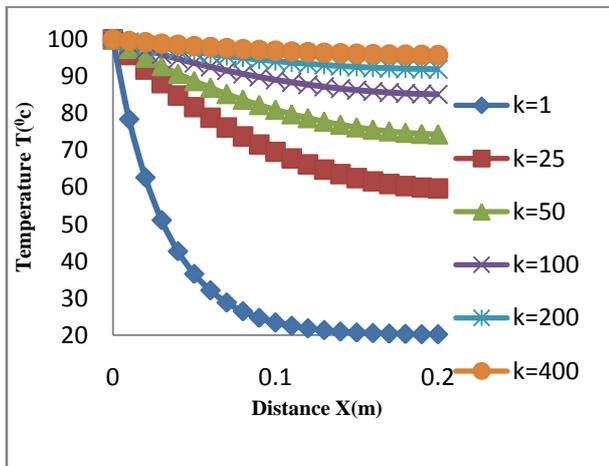
**Fig.10. Temperature Profile for Convective Tip.**
