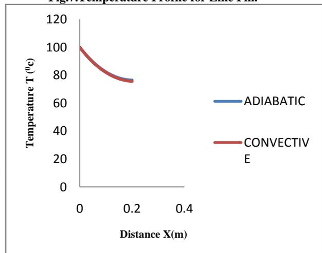
Fig.8. Temperature Profile for Carbon Steel Fin.
