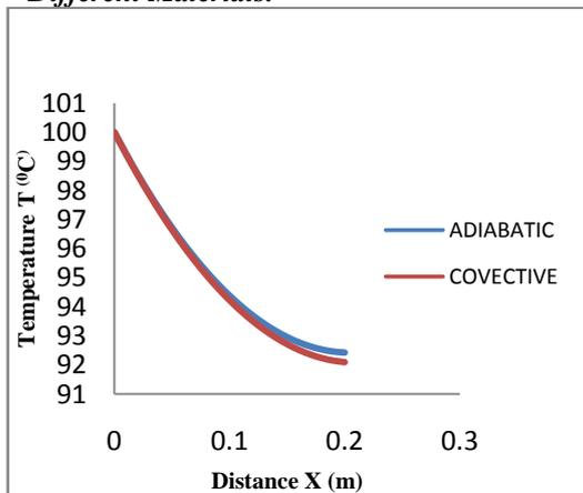
Fig.5. Temperature Profile for Alluminium Fin.
