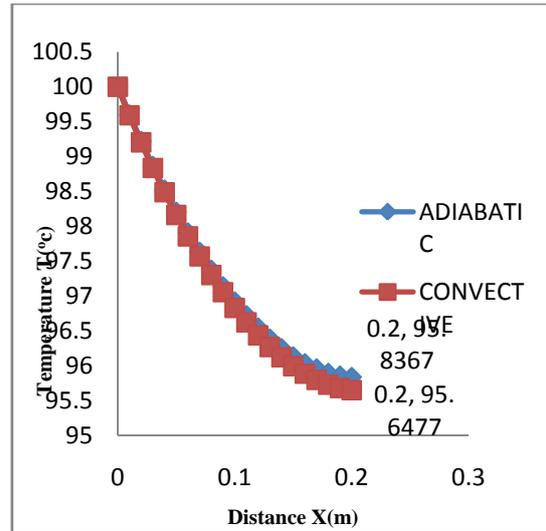
Fig.6. Temperature Profile for Copper Fin.
