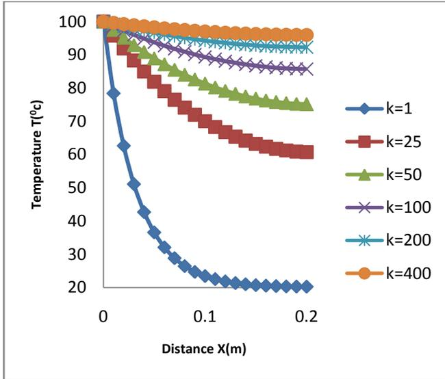
**Fig.9. Temperature Profile for Adiabatic Tip.**
