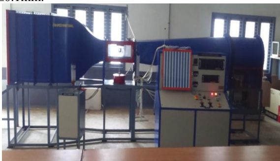
Fig. 2 Photographic View of Low Speed Wind Tunnel.
