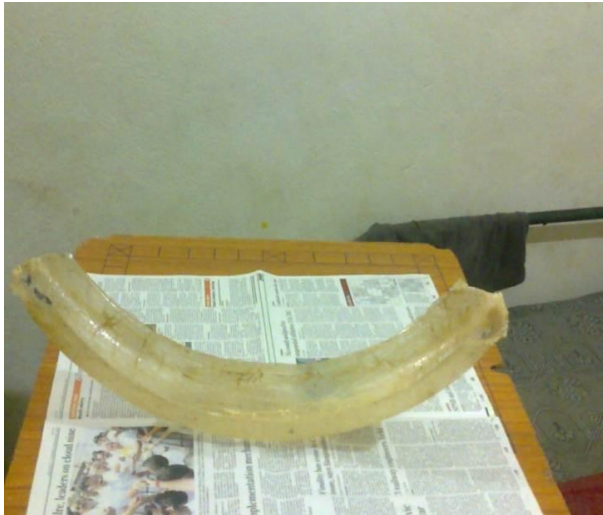
Fig 3. A View of Mudguard produced using wooden Dies
