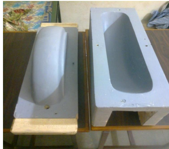
Fig 2. Wooden mould for fabricating mudguard
