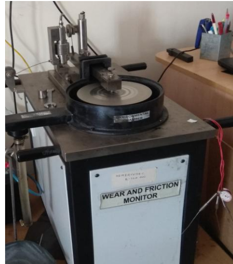
Fig 3 Pin-on disc apparatus
