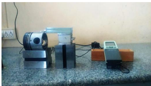
Fig. 2. Surface Roughness Measuring Test Equipment
