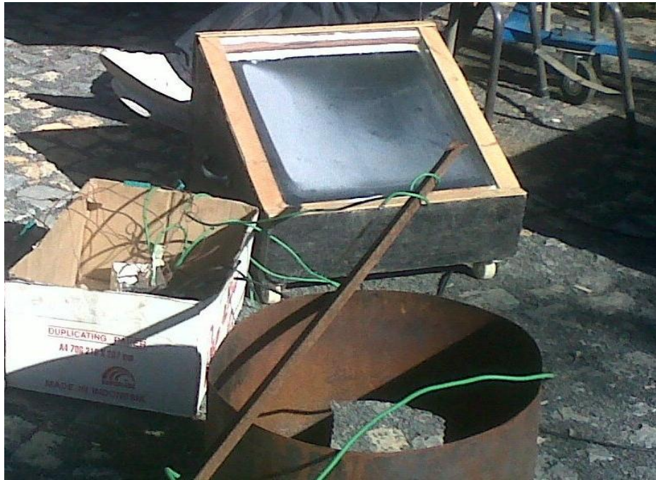
Figure 3 Solar Cooker with black coated box
