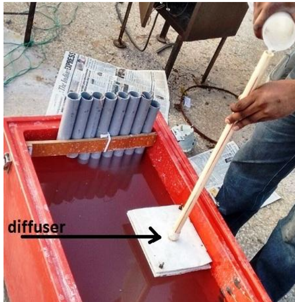
Fig. 4: Formation of NCZ using diffuser
