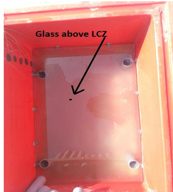
Fig. 5: Solar Pond with Glass above LCZ
