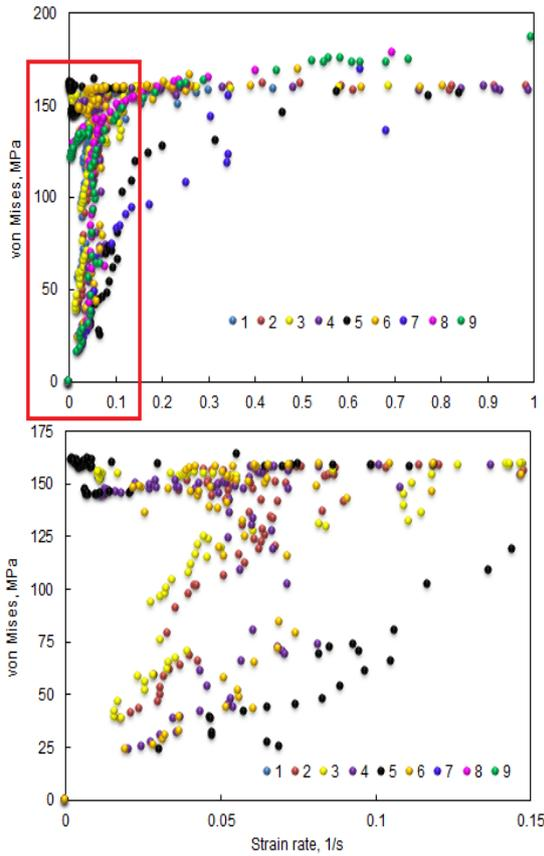
Fig. 5: Effect of strain rate on von Mises stress for all trials.
