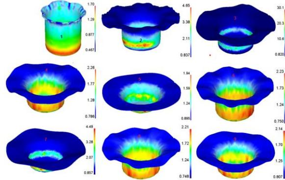
**Fig. 11: Effect of process parameters on the surface expansion ratio.**
