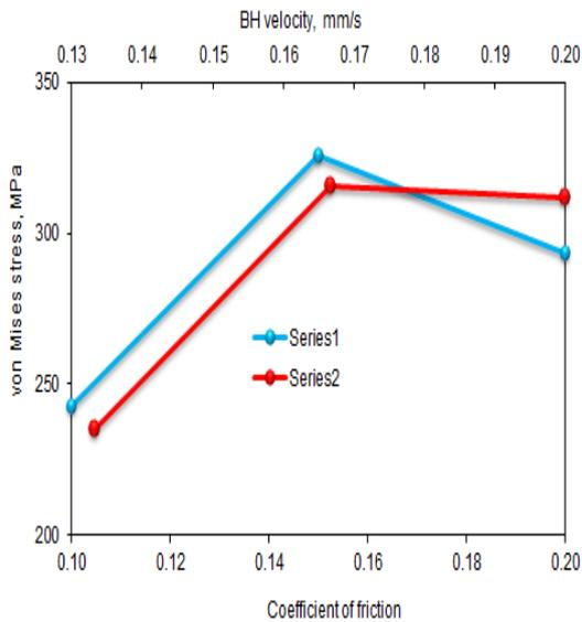
Fig. 6: The von Mises stress as a function of COF and BH velocity.
