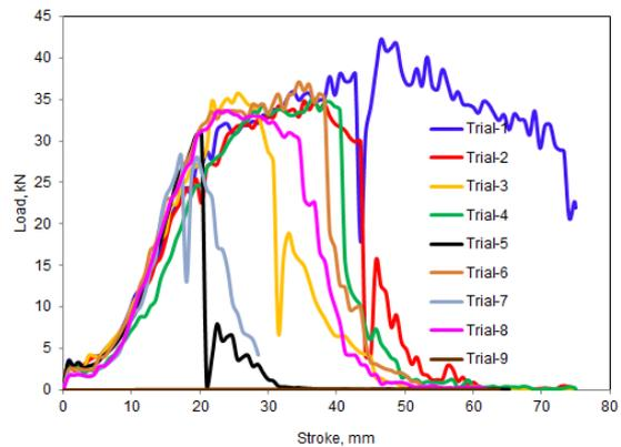
Fig. 8: Applied load as a function punch stroke.
