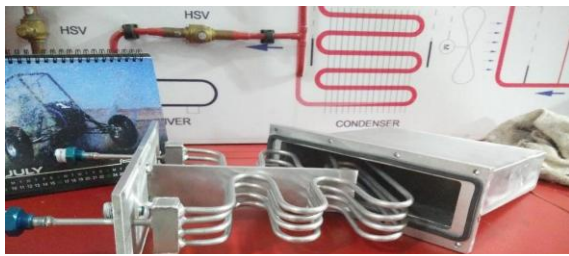
Figure 3: The designed water cooled condenser
