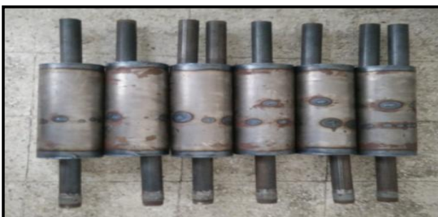
Figure 4: Manufactured all Six Arrangement of Muffler
