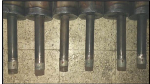
Figure 5: Punching(Marking) at Inlet Pipes of Muffler
