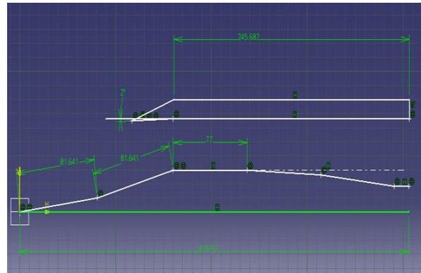
Figure 1 Inlet configuration with 2° cowl deflection angle (All dimensions are in mm)
