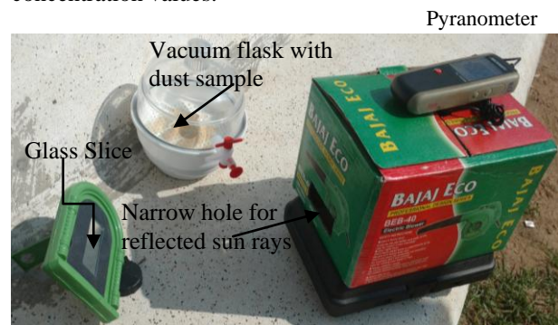
Figure 2: Reflectivity measurement arrangement
