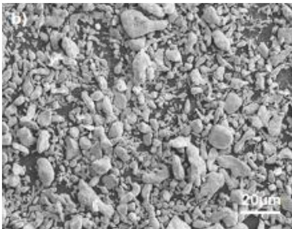
Fig 4: SEM Image of AA 7068 Powders after 20 Hours of Milling
