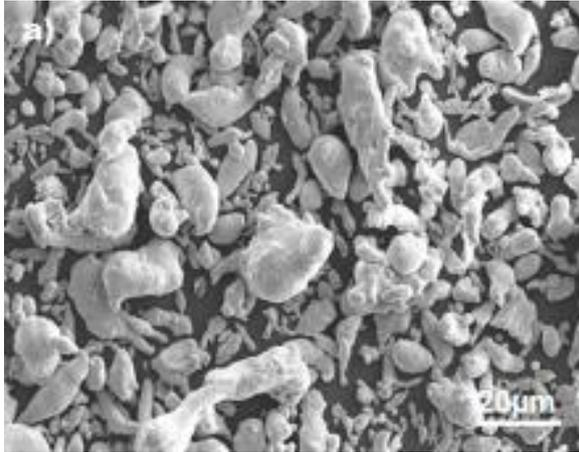
Fig 3: SEM Image of AA 7068 Powders before Milling
