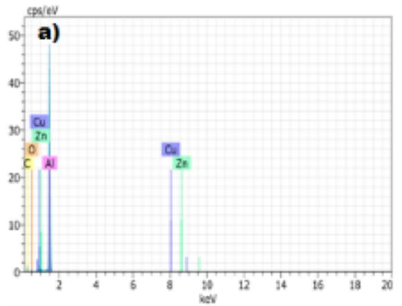
Fig 6: EDAX Pattern for AA 7068 Powders before Milling
