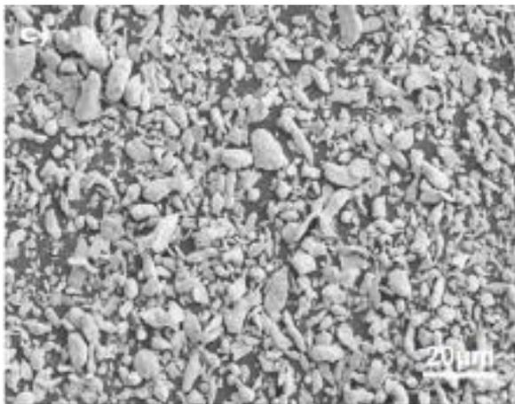
Fig 5: SEM Image of AA 7068 Powders after 40 Hours of Milling
