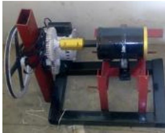
**Fig 2: Fabricated Ball Mill**
