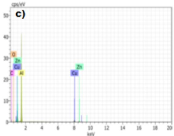
Fig 8: EDAX Pattern for AA 7068 Powders after 40 Hours of Milling
