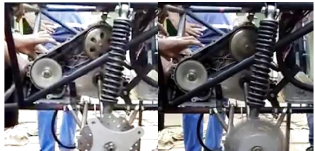
Fig 3: CVT disengaged state (Left) and engaged state (Right)
