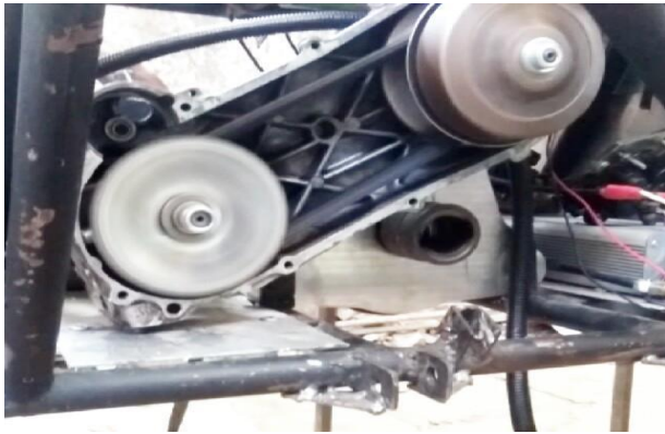
Fig 4: CVT at highest gear (lowest gear ratio – 0.85:1)
