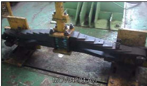
Fig 14: Leaf spring at final stage (fully loaded)
