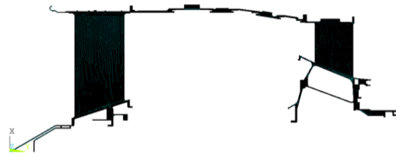
Figure 1: Finite element model of fan casing
