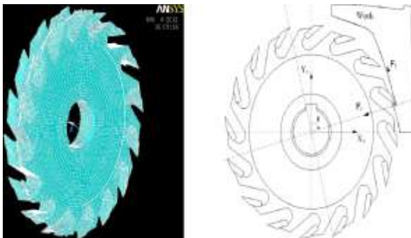
Figure 0.6 Meshing of Special Milling Cutter designed for Leather Industries & Forces acting on milling cutter.
