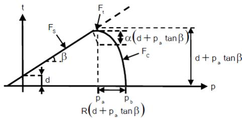
Figure 1 Shows the Modified Drucker-Prager cap model
