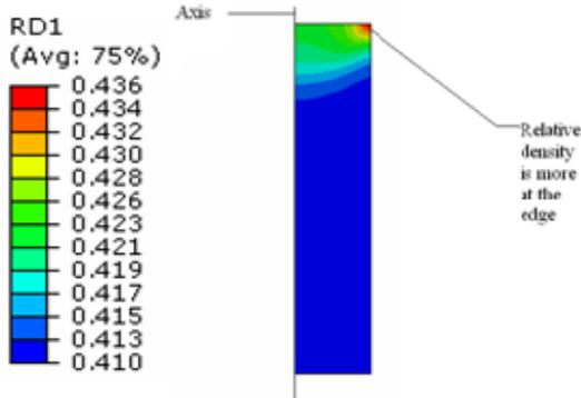
Figure 7 The variation of Relative Density for 5mm Compaction
