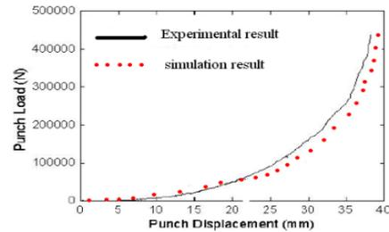
Figure 5 The load vs. Displacement of the simulation and the experimental given in the literature are matching
