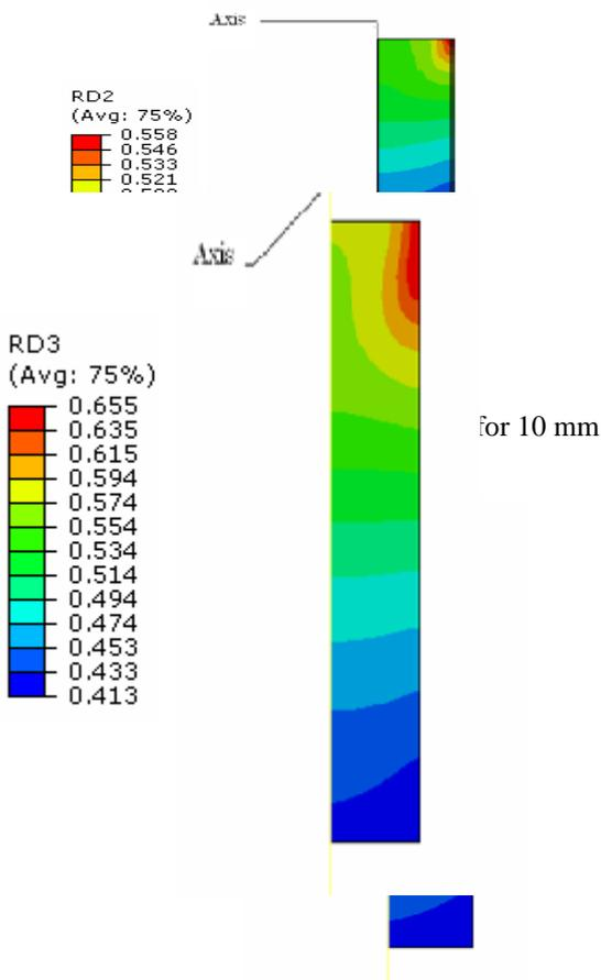
Figure 9 The variation of Relative Density for 15 mm Compaction
