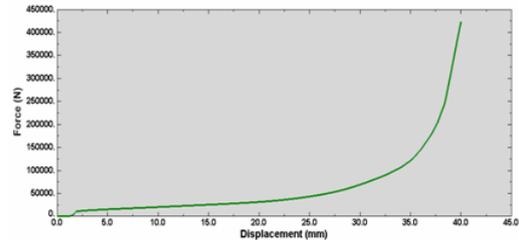
Figure 6 The punch load vs. displacement results of the simulation
