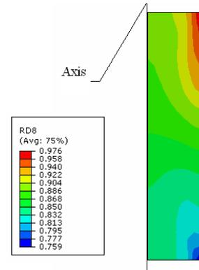
Figure 10 The variation of Relative Density for 40 mm Compaction
