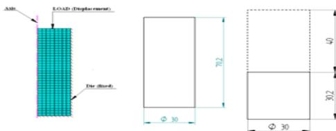
Figure 2 Boundary condition Figure 3 Before Compaction Figure 4 After Compaction
