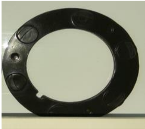
Fig. 9 Old damper at uniform load distribution
