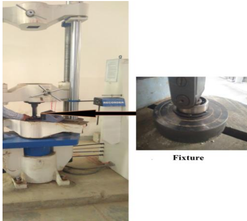
Fig. 20 Experimental setup on UTM
