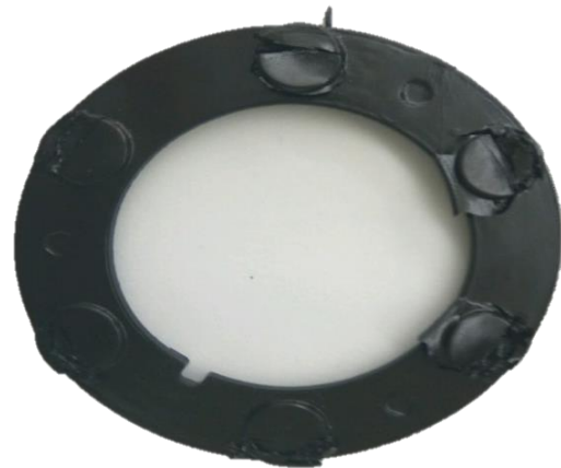
Fig. 6 Old damper at uneven load distribution
