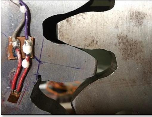
Fig 4: Pinion Tooth with 5mm Crack
