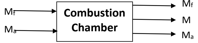
Figure 2. Mass Balance in Combustion Chamber
