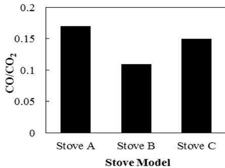
Fig 9: CO/CO<sub>2</sub> emission in flue gas
