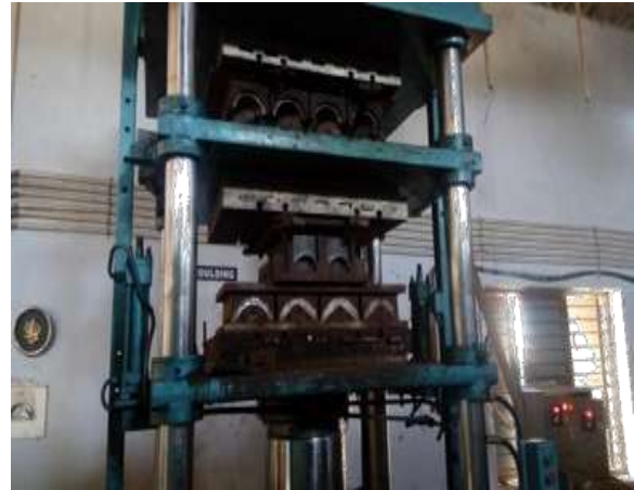
Fig 2. Hot molding/press setup
