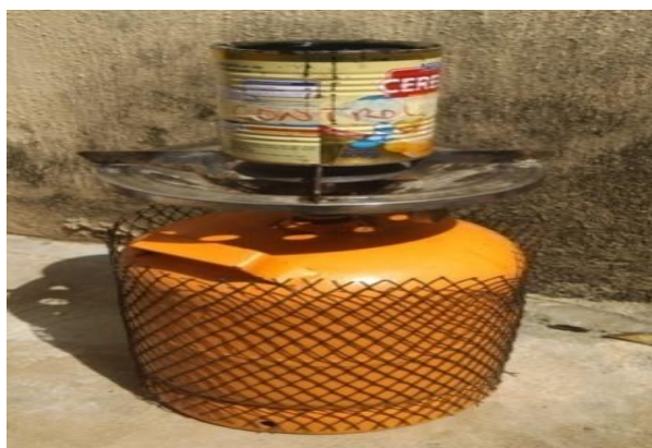
Plate I: A gas unit with the steel container for heating the bituminous samples
