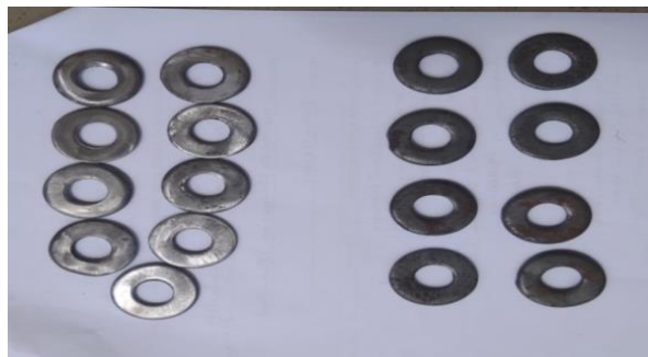
Plate II: Cleaned and coated annular disk coupons for the test.
