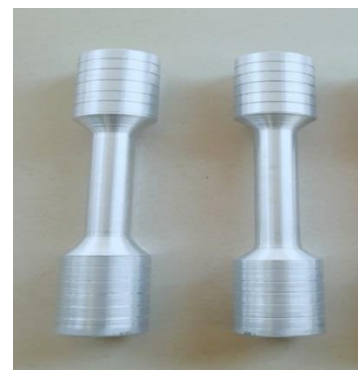
Fig. 5 Specimen for Tensile Test
