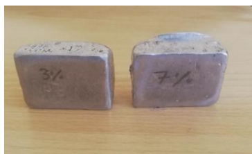
Fig. 3 Specimen for Hardness Test
