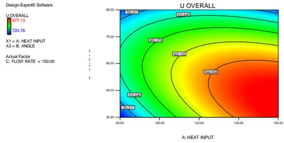
**Fig 5: Counter plot for  $U_{Overall}$  concerning heat input and angle**
