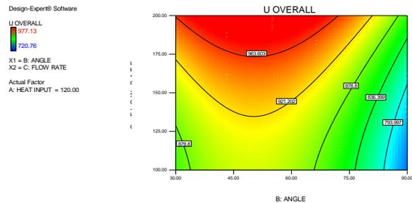
**Fig 7: Counter plot for  $U_{overall}$  concerning angle and flow rate**
