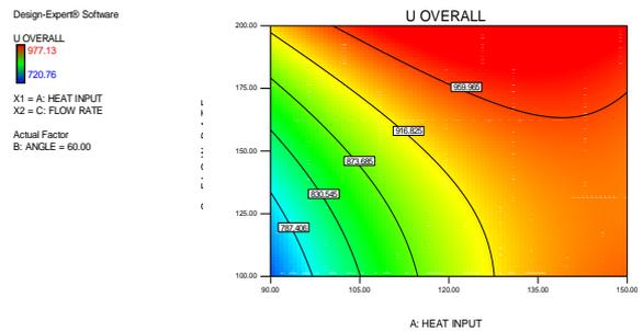
**Fig 6: Counter plot for  $U_{overall}$  concerning heat input and flow rate**
