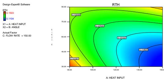
**Fig 2: Contour plot for Rth concerning heat input and angle**
