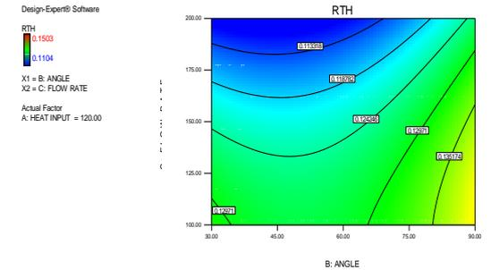
**Fig 4: Contour plot for Rth concerning angle and flow rate**
