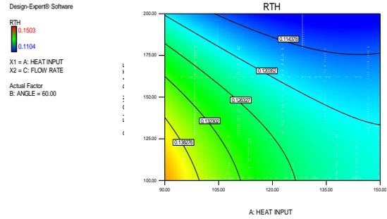
**Fig 3: Contour plot for Rth concerning heat input and flow rate**
