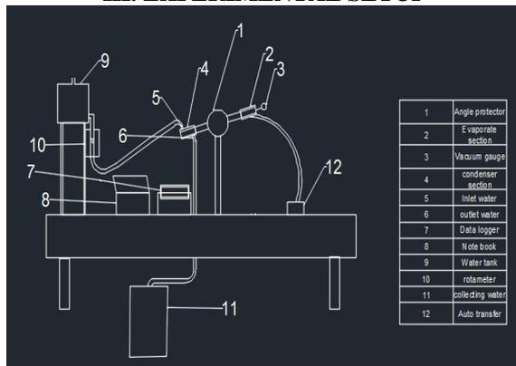
**Fig 1. The layout of the experimental setup**
