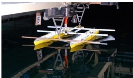
Fig 3: Model ship resistance test
