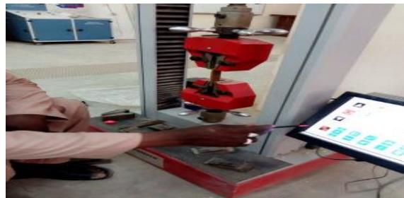
Plate VII: Load Application for Tensile Strength
