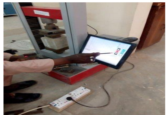
Plate VIII: Load Application for Compressibility & Recovery Test
