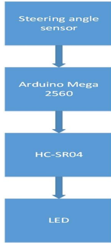
Fig. 11 The measurement processes of the warning system
